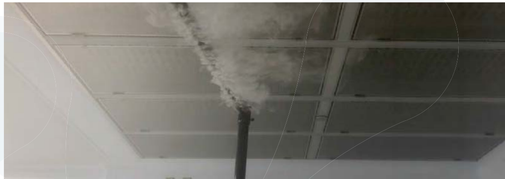
Figure 4 Glycol-based Tracer Particle Generator Note: Beneath HEPA filters HVAC is Off
