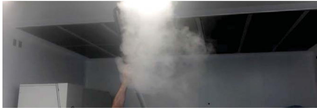
Figure 3 Nitrogen and water “Cleanroom Fogger” beneath a florescent light (dead zone) the smoke sinks, giving the false impression of unidirectional airflow
