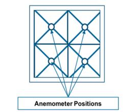
It is important to retain air velocity measurements for each grid location of each HEPA filter. Comparisons to the initial test data should be made for every successive test. HEPA filters are the last line of defense in critical high risk operations. Filters can be damaged or compromised by regular operations, decontamination practices or other testing methods such as filter integrity testing.
