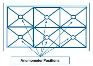
600 mm x 600 mm (2 ft x 2 ft) HEPA Filter: 4 Point Air Velocity Measurements
